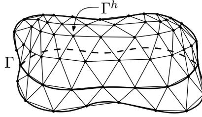
FIGURE E.4. Mesh  $\Gamma^h$ , discretization of  $\Gamma$ .
