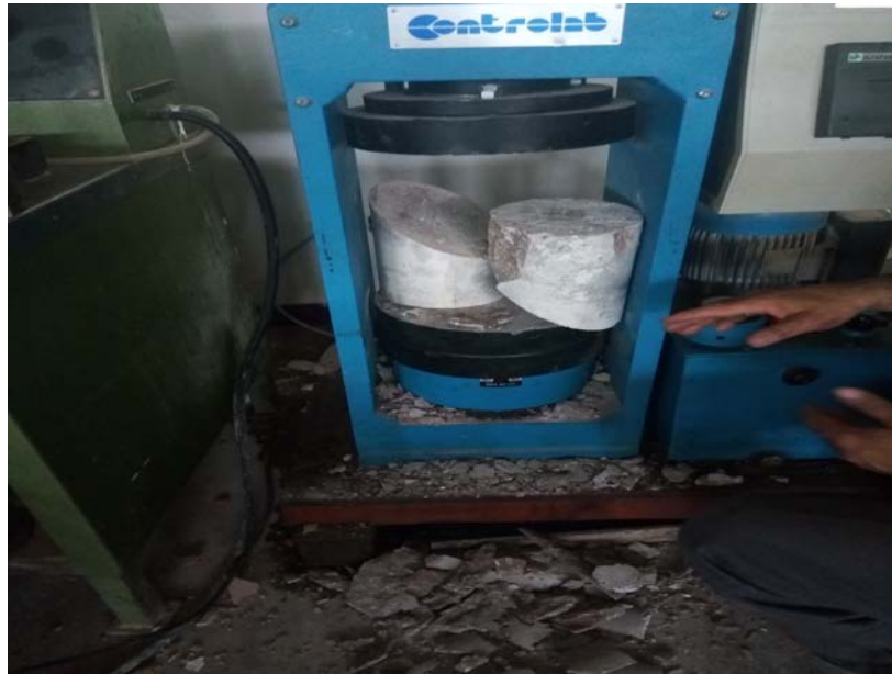
Figure IV.30 : essai de compression.
