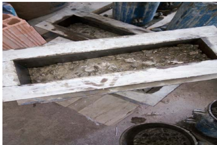
Figure IV.3 : moule 10x10x40cm 3 surface horizontale.
