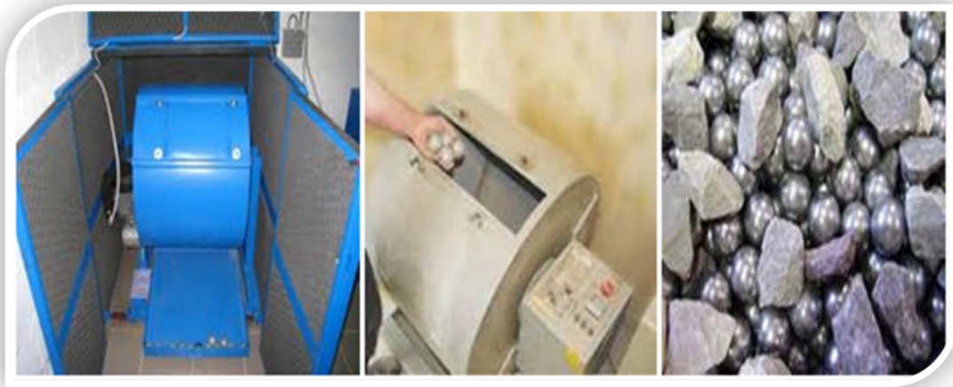
Figure 5.7 : Essai los Angeles [5].
