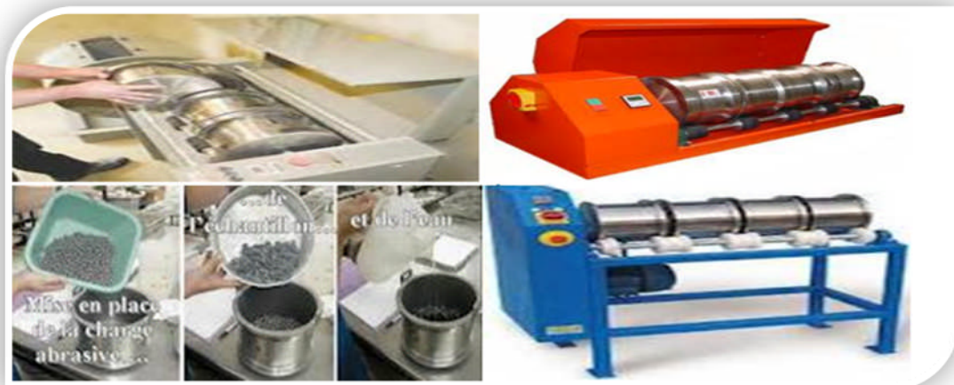
Figure 5.8 : Essai Micro Deval [5].
