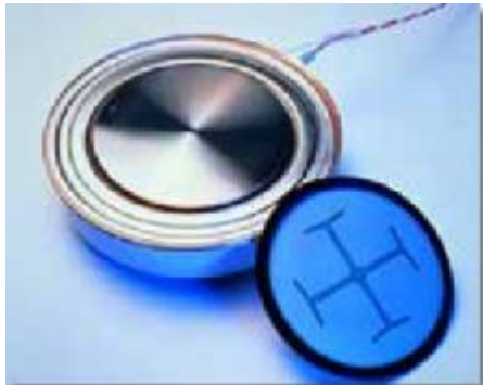
Figure I.18: Thyristor press-pack Figure I.19: IGBT press-pack [Source ABB]
