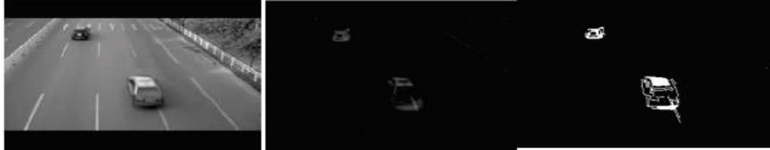
Figure 20. Background subtraction while the execution of the object (cars) counting process. Source. Li et al., (2014, p. 1).
