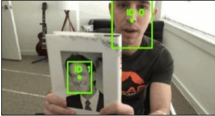
Figure 19. Algorithm for tracking functioning centroids.
