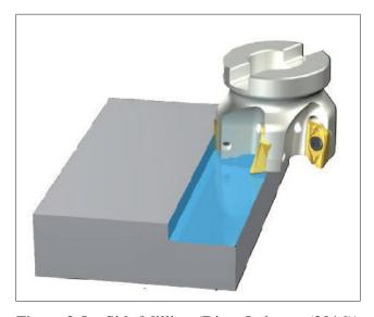
Figure 2.5 Side Milling (DirectIndustry (2016))
