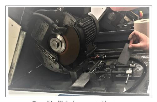
Figure 2.2 Work pieces are cut with wet saw
