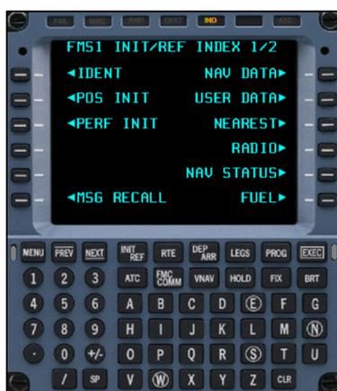
Figure 3.11 Control Display Unit (CDU) du CMA-9000 FMS
