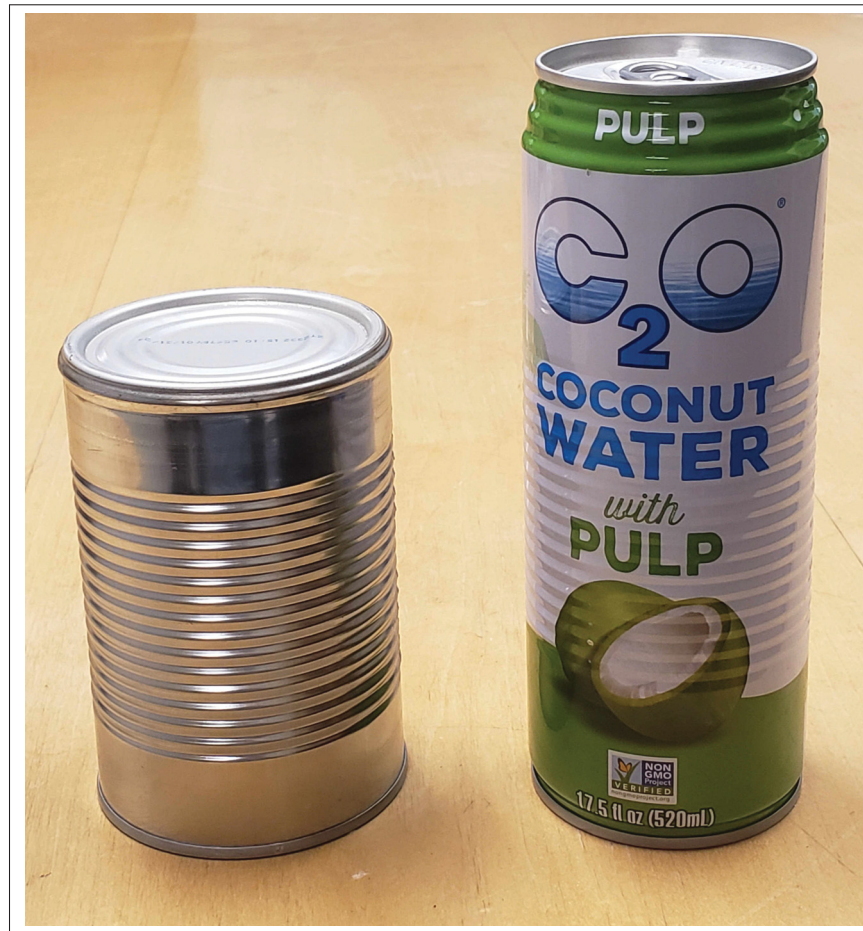
Figure 4.9 Two objects that were confused during the evaluation made by the combined machine learning agents: a can of peas (shown on the left, its label was removed after the experiments) and a coconut water bottle – Conversely to Fig. 4.2, these visually-different objects are however similar from a tactile sensing perspective: they are both very rigid, they both have a smooth but corrugated surface, they have a similar radius (at the location where they were touched during the exploration phase) and a perceived deformation pattern (evolution of the contact area over time), when compressed, that looks alike
