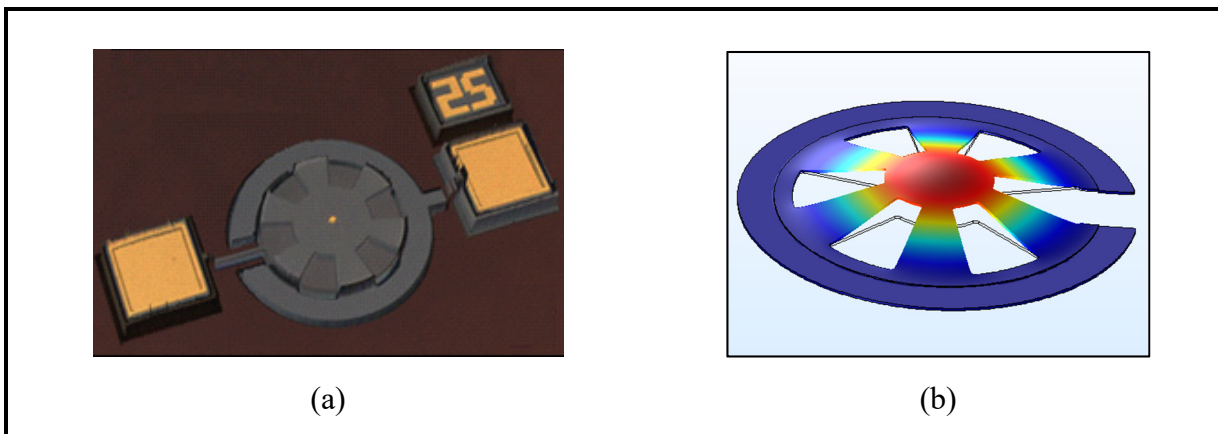
Figure 2.9 (a) 3D view of the real micro-resonator obtained by the Olympus LEXT OLS4000 Confocal microscope, (b) Eigenfrequency FEM COMSOL simulation
