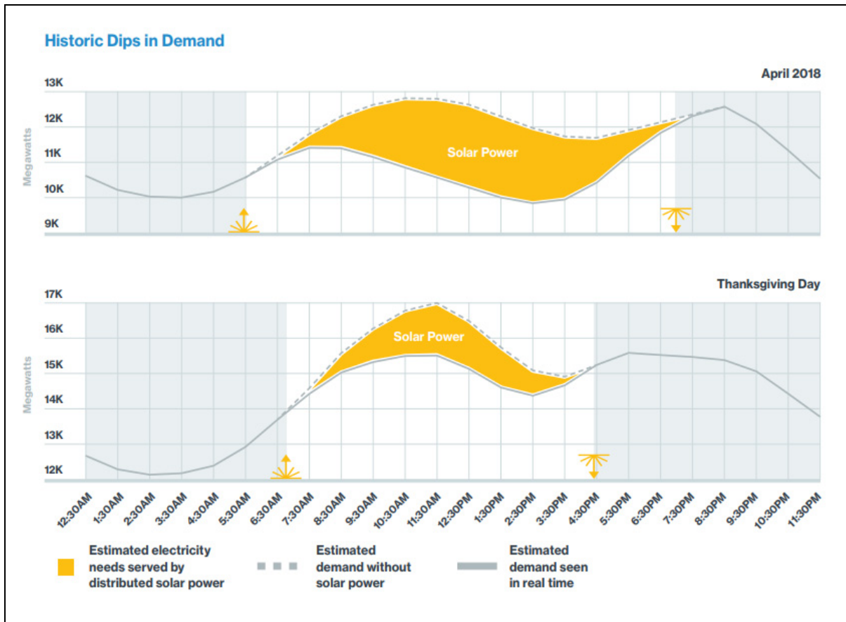
Figure 1.19 Solar energy effect to daily load profile
