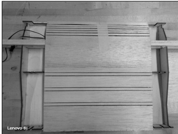
Figure 5.10 Central section of the wing corresponding to the MC system
