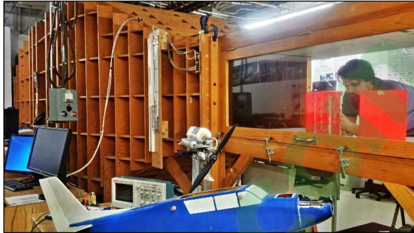
Figure 3.11 LARCASE Price-Paidoussis subsonic wind tunnel
