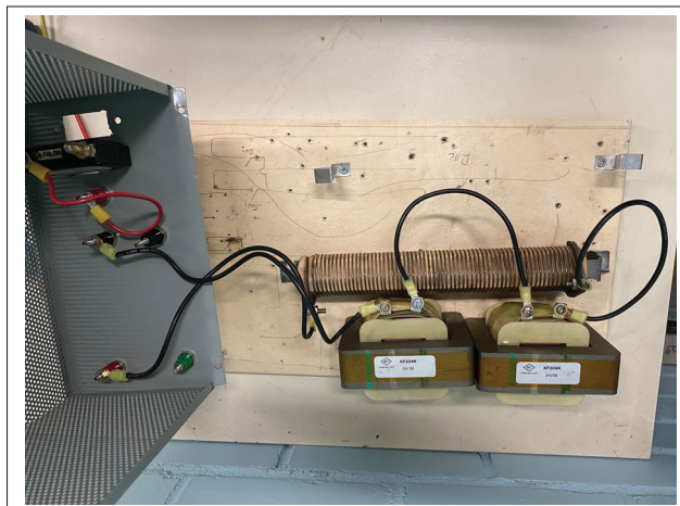
Figure 6.7 Load used during experiments (uncovered)
