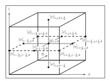
**Figure 4.1** Spatial distribution of model variables and constants in the Arakawa C-type grid, for which  $\phi = f, S, K_{w}, K_{T}$  and  $\psi = w, T, b, TKE$ .
