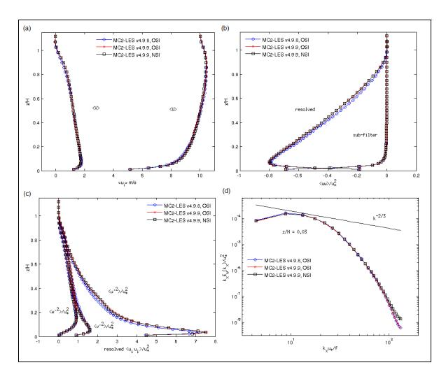
Figure 4.5 Ensemble averaged (a) streamwise and spanwise velocity components, (b) resolved and SGS normalized  $\tau_{13}$  stresses, (c) resolved velocity variances and (d) surface layer energy spectra.
