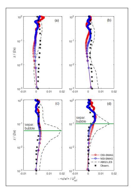
**Figure 4.12** Time and spanwise averaged normalized  $\tau_{13}$  stress at the (a) upslope, (b) hill crest, (c) downslope and (d) base positions of the H3 ridge.
