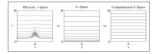
**Figure 1.2** Height of the computational levels in physical z-coordinates (left), Gal-Chen η-coordinates (middle) and computational Z-coordinates (right). Leuenberger et al. (2010).
