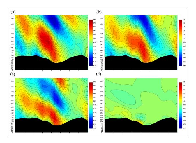
**Figure 3.4** Vertical velocity cross-sections of four climate-states with the same mean wind speed of 7 ms<sup>-1</sup>, wind direction of 225 degrees and positive shear, classified with different Brunt-Väisälä frequencies of (a) 0.0091 s<sup>-1</sup>, (b) 0.0137 s<sup>-1</sup>, (c) 0.0174 s<sup>-1</sup> and (d)  $0.022 \text{ s}^{-1}$ , respectively.
