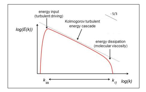
Figure 1.1 Energy spectrum of a well-developed turbulent flow
