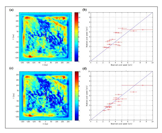
**Figure 3.6** Wind speed (ms<sup>-1</sup>) distribution (left panels) and comparison of modeled versus observed wind speeds (right panels) over the Whitehorse area, obtained with the OC+OSI combination implemented in (a)-(b) MC2 v4.9.6 and (c)-(d) MC2 v4.9.8, respectively.
