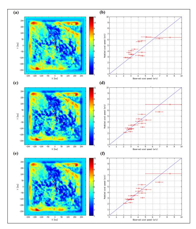
**Figure 3.7** Wind speed (ms<sup>-1</sup>) distribution (left panels) and comparison of modeled versus observed wind speeds (right panels) over the Whitehorse area, obtained with the (a)-(b) NC+OSI, (c)-(d) OC+NSI and (e)-(f) NC+NSI combinations implemented in MC2 v.4.9.9.
