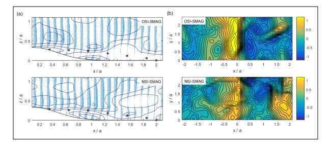
**Figure 4.11** Time-averaged (a) vertical flow field contours and vector depiction at the transverse centerline, with \* representing the observed H3 separation streamline, and (b) horizontal winds  $\overline{u}/U_{ref}$  at  $z \approx 7 \times 10^{-3}$  m a.g.l., the first internal momentum level.
