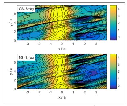
**Figure 4.8** Time averaged wind fields (ms<sup>-1</sup>) at 10 m a.g.l. over the symmetric Gaussian ridge with both SI schemes combined with the Smagorinsky turbulence closure.
