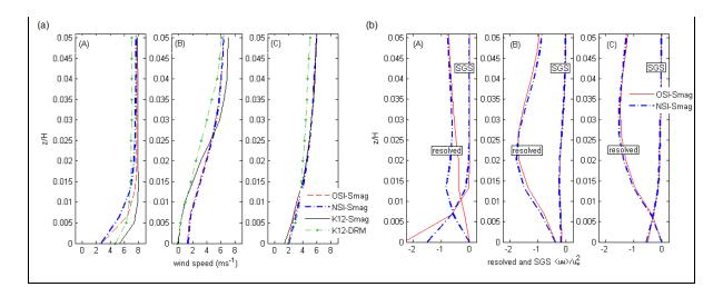
Figure 4.7 Time and span-wise averaged (a) wind speed and (b) resolved and SGS parts of the  $\tau_{13}$  stress within the surface layer at the [A] hill crest, [B] downslope lee-side and [C] base valley along the Gaussian ridge.
