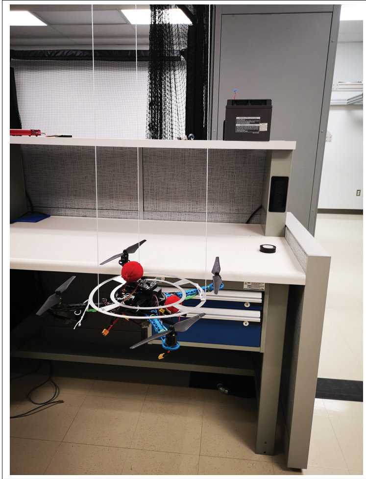
Figure 2.7 Measurement of Mass Moment of Inertia along z-axis.
