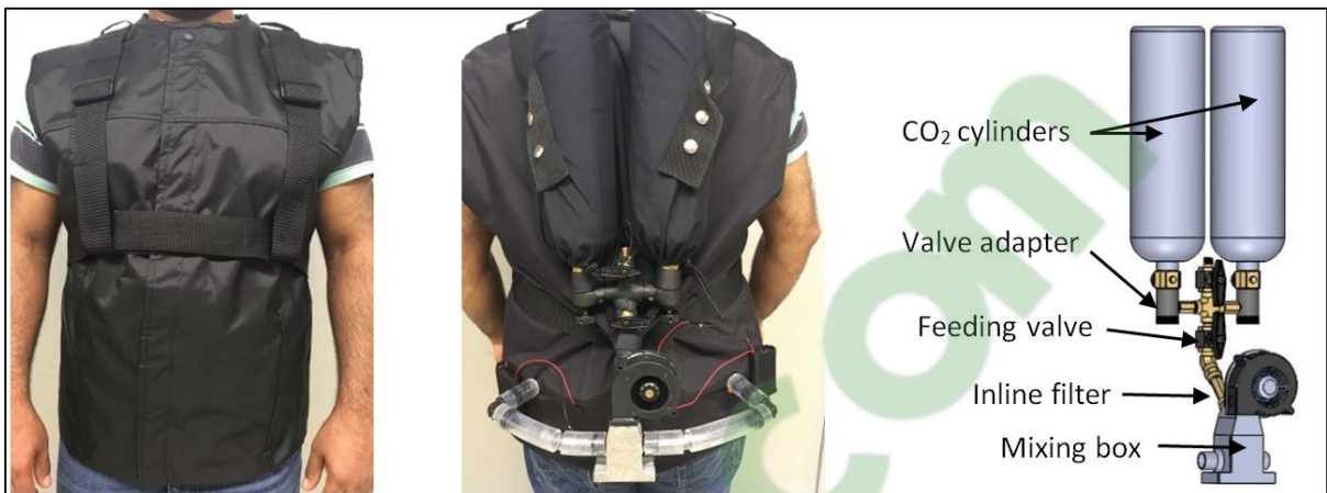
Figure 6.1 Front view, back view, and the air treatment system of the cooling garment.
