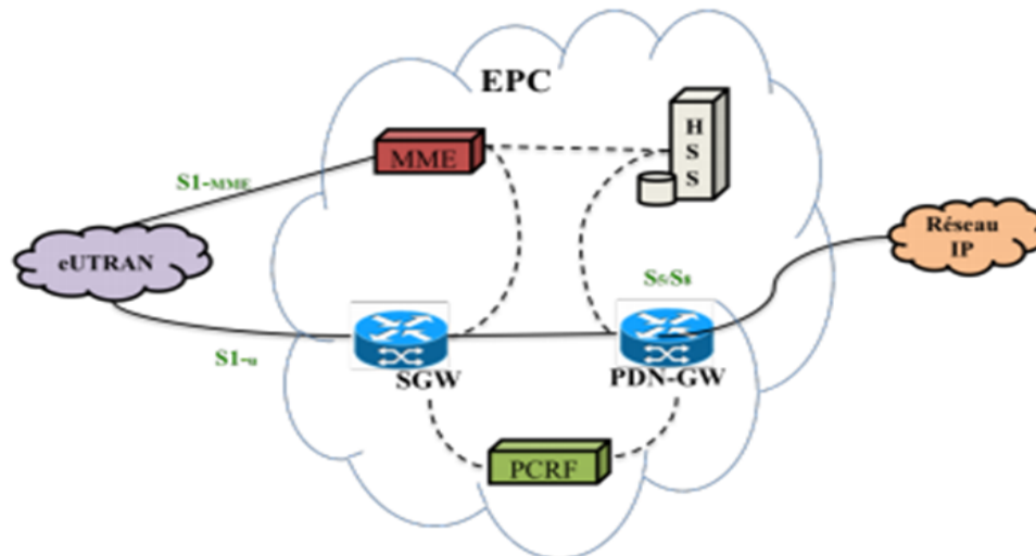
FIGURE I.3 – Architecture d'EPC (Evolved Packet Core)
