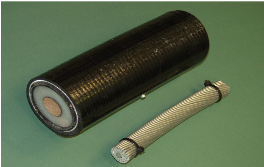
Figure 2-2 Thick underground cable next to smaller overhead conductor (Photo courtesy of Georgia Transmission Corporation)
