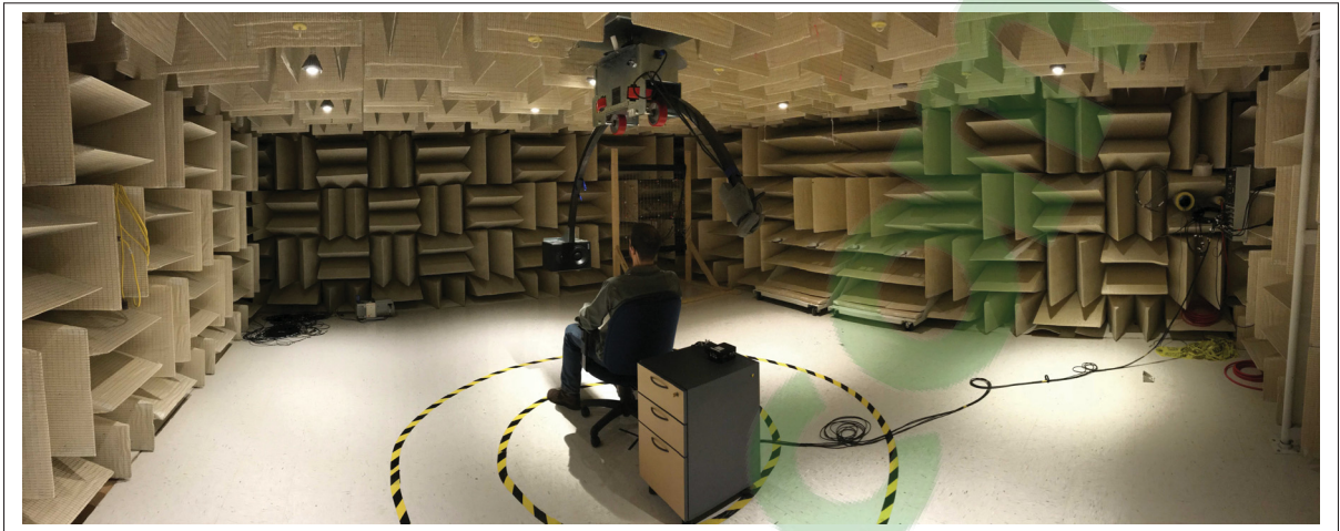
Figure 4.2 Semi-anechoic room used for tests with the earpieces
