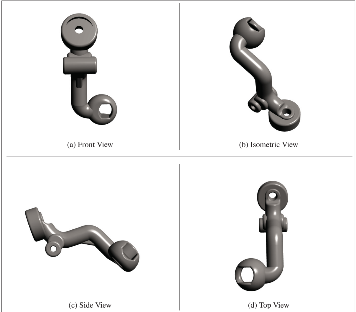
Figure-A II-12 Lever 3D rendering views
