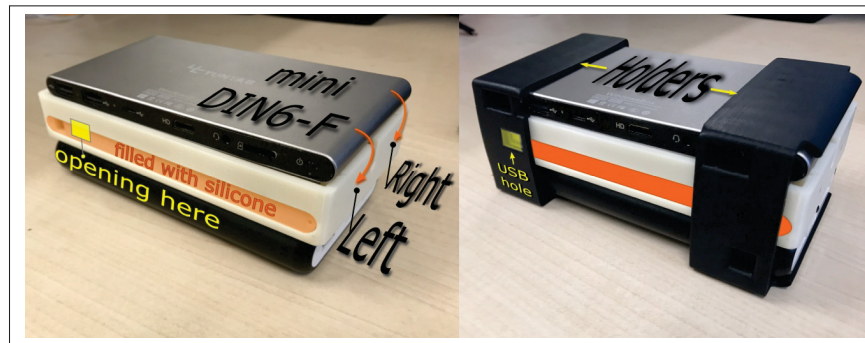
Figure-A III-1 Main Work: USB opening - Silicone filling - Connectors holes (left) and final assembling with the two holders (right)
