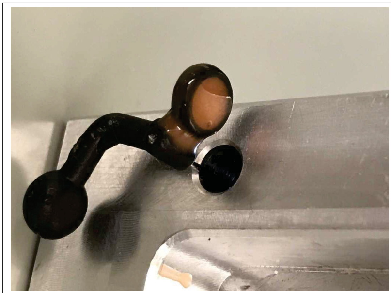
Figure-A II-16 Lever filled with silicone
