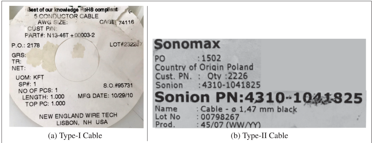
Figure-A II-5 Examples of cables used in the prototypes
