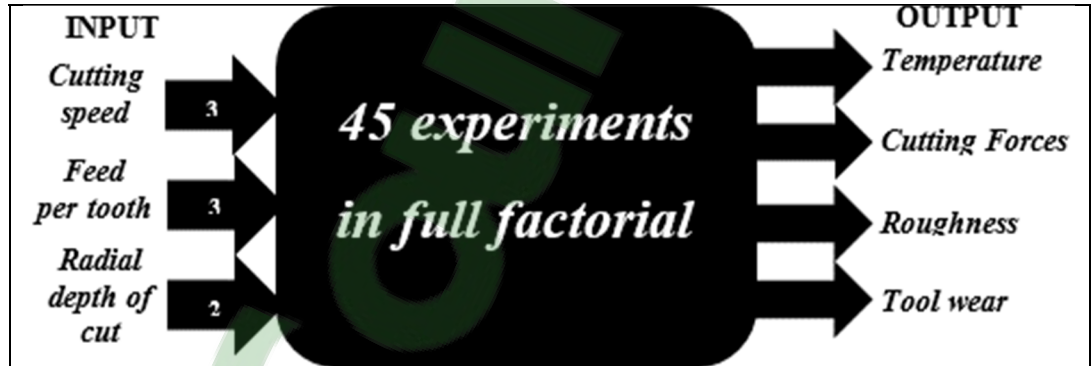
Figure 2.2 Sketch of final DOE with inputs and outputs
