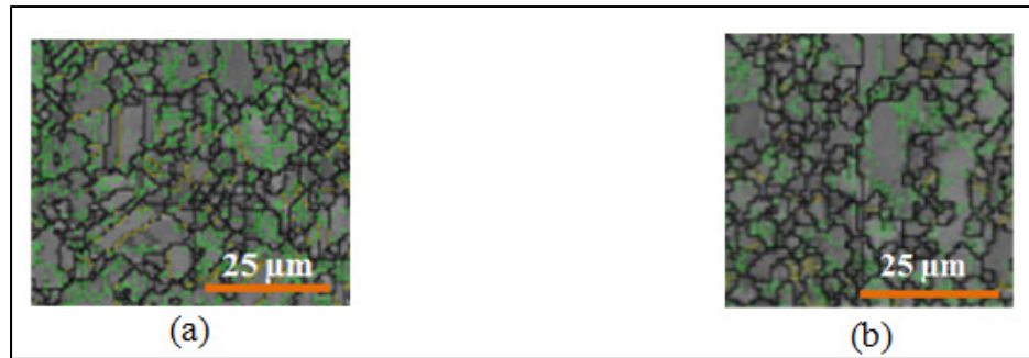
Figure 2.14 EBSD grain boundary map of the LFWed sample#4; (a) 0.6 mm and (b) 0.2 mm from the weld interface showing grain boundary bulging.
