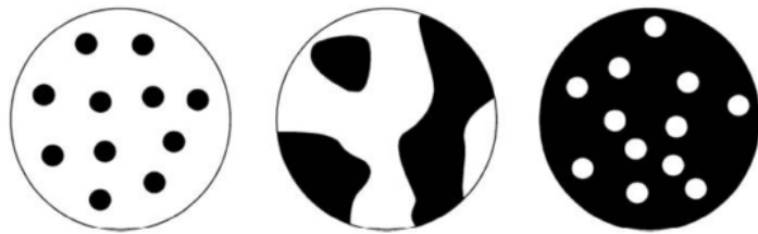
FIG. 1.1 Evolution of a blend morphology as a function of concentration [1]
