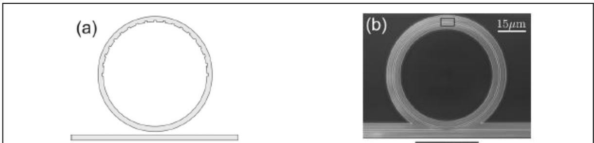
Figure 2.5 a) Schematic of the ring with integrated DBR. The DBR is realized by modulating the top half of the ring waveguide. b) SEM image of the fabricated device prior to top cladding deposition
