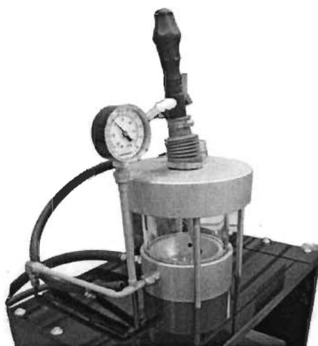
**Fig 2.1** Arc-melting machine
