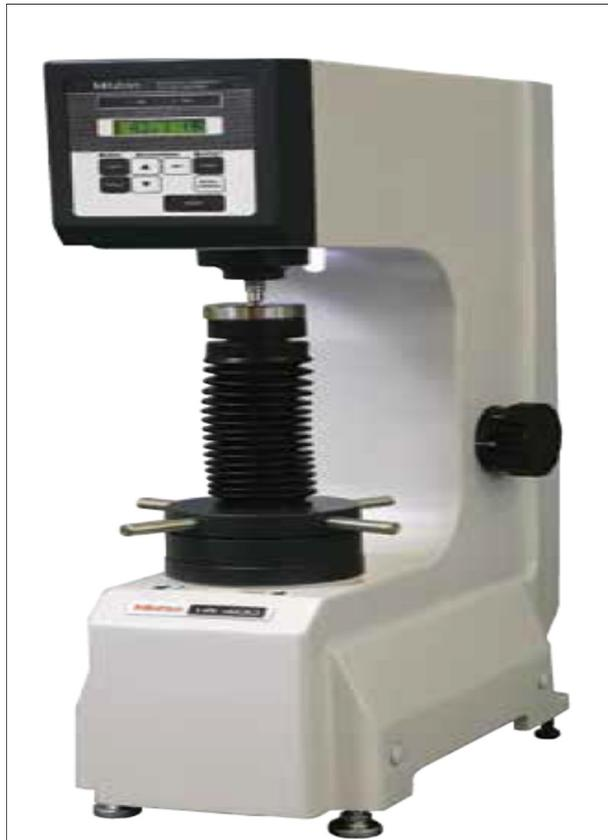
Figure 2.11 Mitutoyo Rockwell hardness machine
