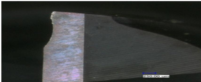
Figure 3.14 Image of tool wear when cutting 410 (50×) Cutting Speed at 150m/min and feed rate at 0.1 mm/tooth
