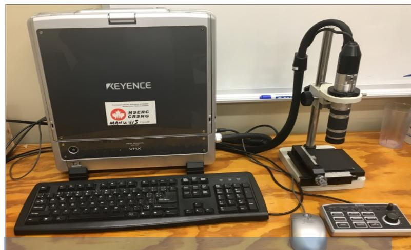
Figure 2.7 Digital microscope KEYENCE, VHX-500F
