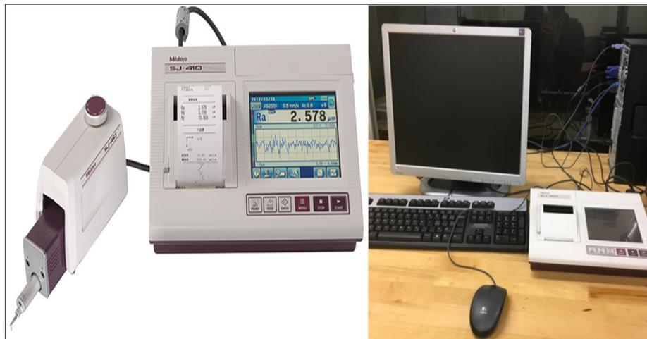
Figure 2.9 Mitutoyo measured Surface Quality testing machine
