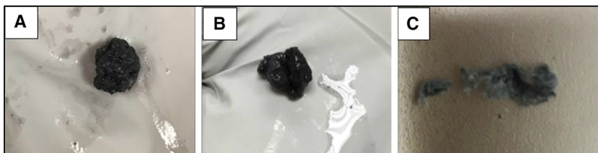
Figure 4.2 Final shape of A Onyx, B 25%-ethanol mixture and C 50%-ethanol mixture after injection in a saline solution bath and polymerization. Note the non-cohesive aspect of 50%-ethanol mixture (C)
