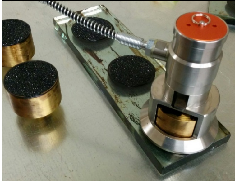
Figure 3.1 Pull-off test adhesion device used : automatic portable Elcometer adhesion tester
