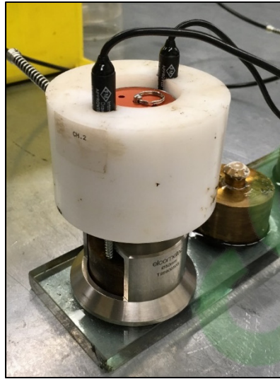
Figure 3.5 Modification of the pull-off test device to include two LVDT for displacement measurements
