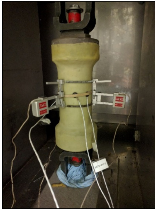
Figure-A VI-2 Apparatus used for complex modulus measurements: latex membrane was used to prevent water loss during testing
