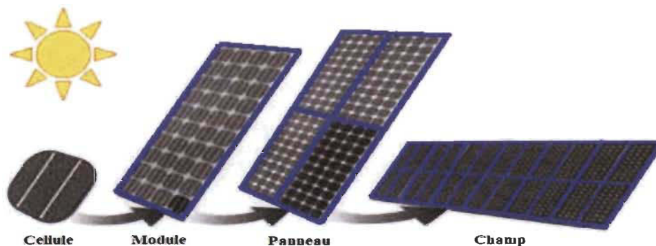
Figure 1.3. Configuration des cellules photovoltaïques [38]
