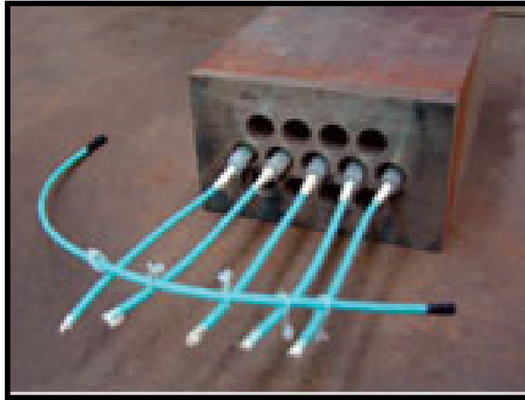
Figure 1.6 Plug installation in explosive expansion ( www.tei.co.uk )
