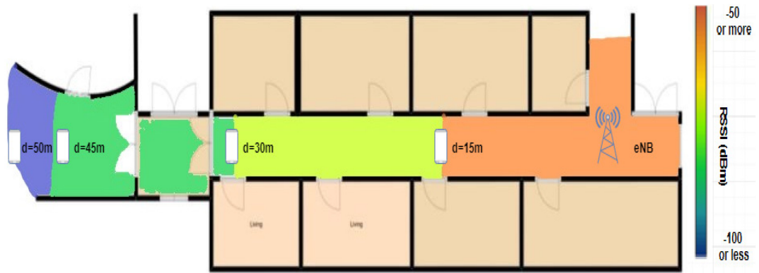
Figure 46: Coverage of LTE mobile platform for an indoor scenario in terms of RSSI.
