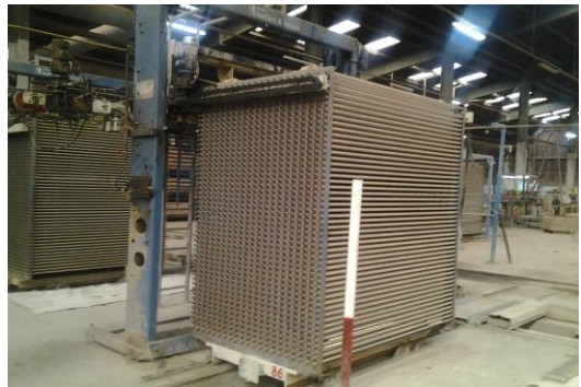
Figure I.2 : Le bras mobile de manutention.
