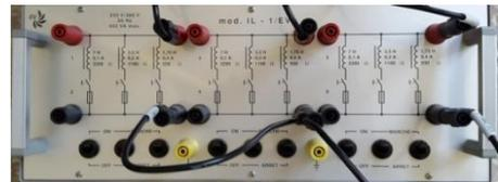
Figure III.1: Inductance variable (MAX  $R=314\ \Omega$  ;  $L=1\text{H}$ )
