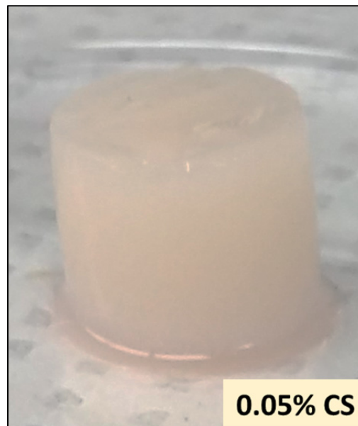
Figure 4.34 Photograph of chitosan-based hydrogel with 0.05% CS after 1h of incubation at 37°C
