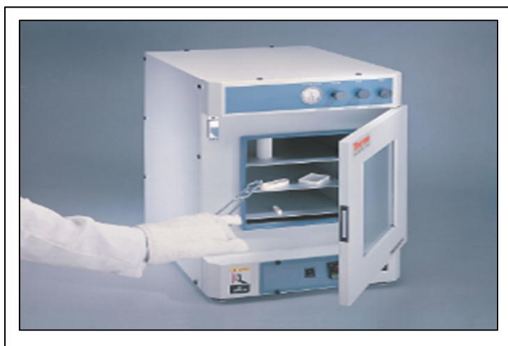
Figure 2.12 Un four sous vide (Thermoscientific)
