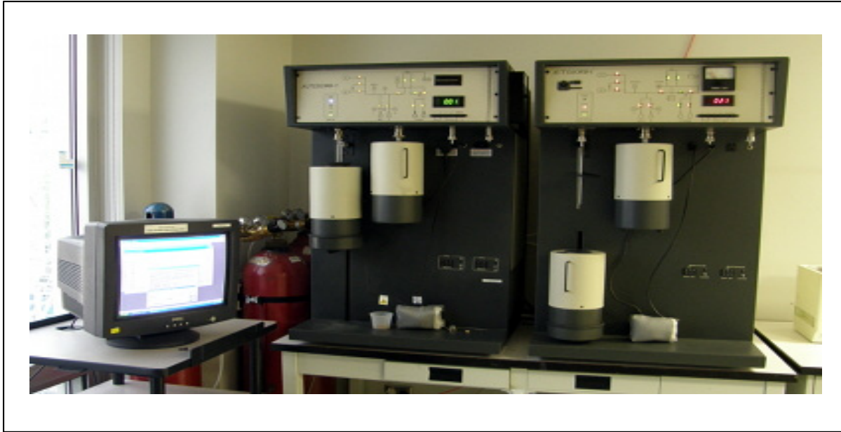
Figure 2.26 Brunauer, Emmett and Teller Instrument (BET)
