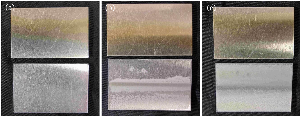
Figure 4-1. Digital images of Al samples (50 mm x 30 mm) treated with N_2 plasma (top) and N_2 - O_2 plasma (bottom) after (a) first pass, (b) second pass, and (c) third pass of plasma treatment.
