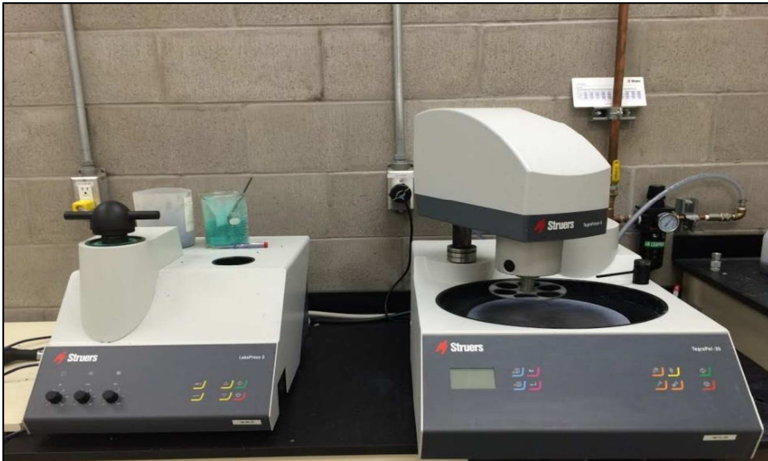
Figure 3-7: (L) Struers LaboPress-3 and (R) TegraForce-5 machines used for mounting and polishing samples for metallography.
