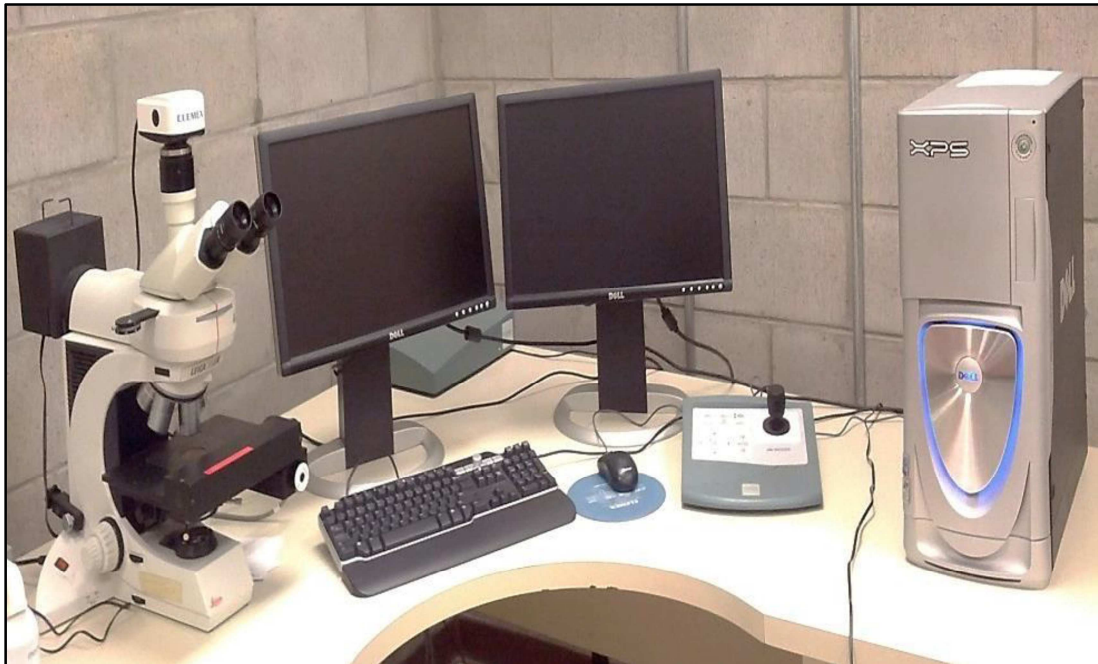
Figure 3-5: Optical microscope-Clemex image analyzer system
