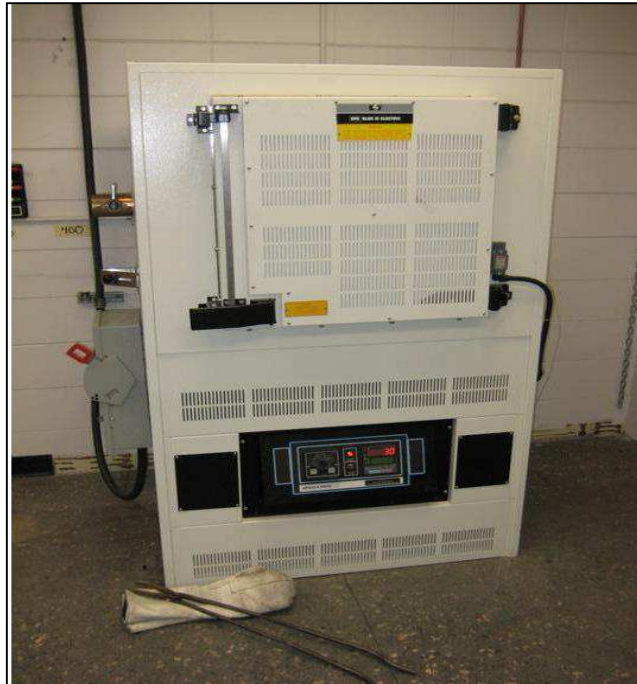
Figure 3-4: Blue M furnace used for heat treatment.
