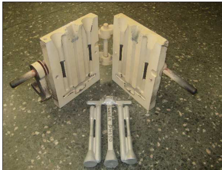
Figure 3-2: ASTM B-108 permanent mold used for casting tensile test bars.
