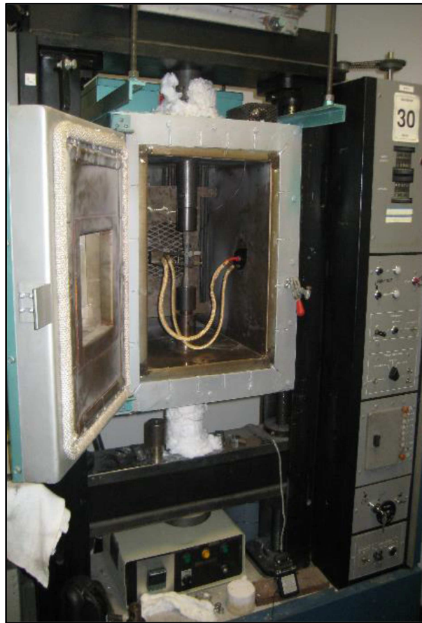
Figure 3-11: Instron Universal Mechanical Testing machine with chamber for high temperature testing.
