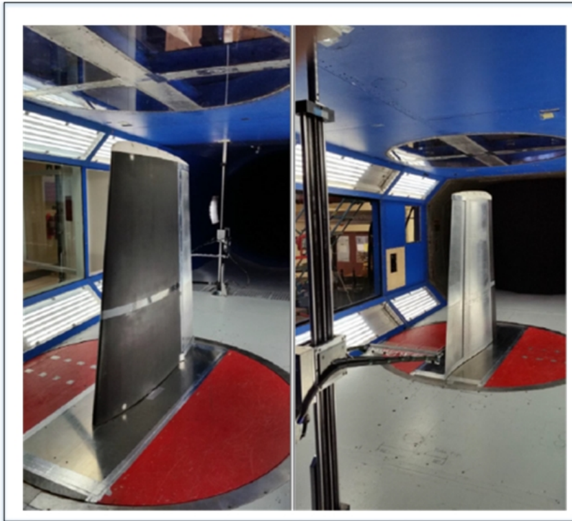
Figure 4.2 CRIAQ MDO 505 project wing model setup in the NRC wind tunnel section
