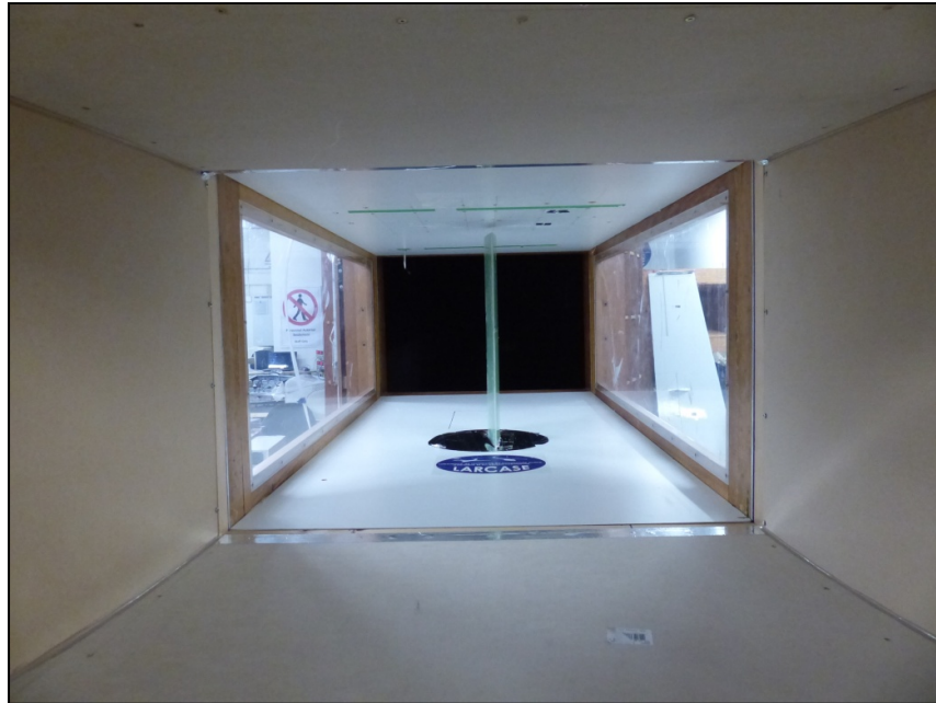
Figure 3.6 Optimized wing model installed inside the test chamber ready for testing
