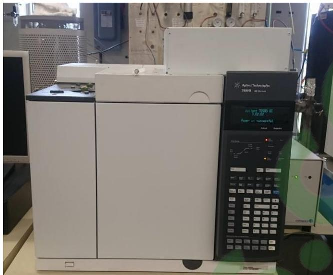
Figure 3.8 Gas chromatograph equipped with a pulsed flame photometric detector (GC- PFPD)
