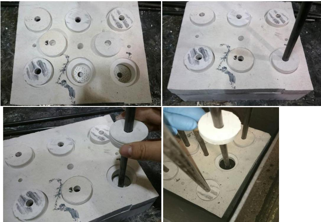
Figure 3.10 The new crucible with 6 sample holders and water connections
