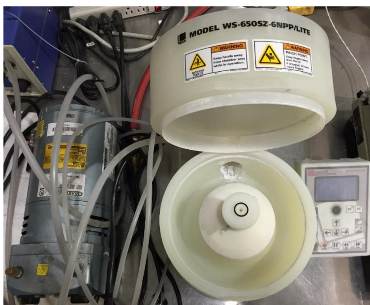
Figure 3. 2 Photograph of Single Wafer Spin Processor
