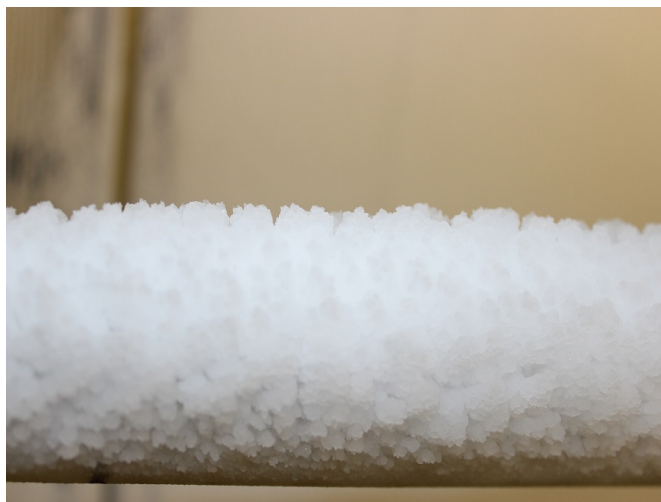
Figure 2-3: Hard rime on a conductor in the experiment
