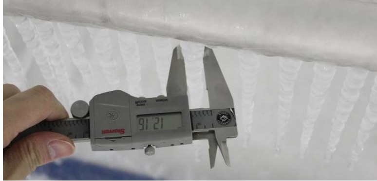
Figure 4-6: Diameter measurement of icicles.
