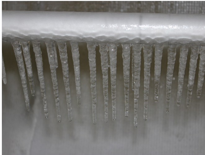
Figure 2-1: Glaze on a conductor in the experiment
