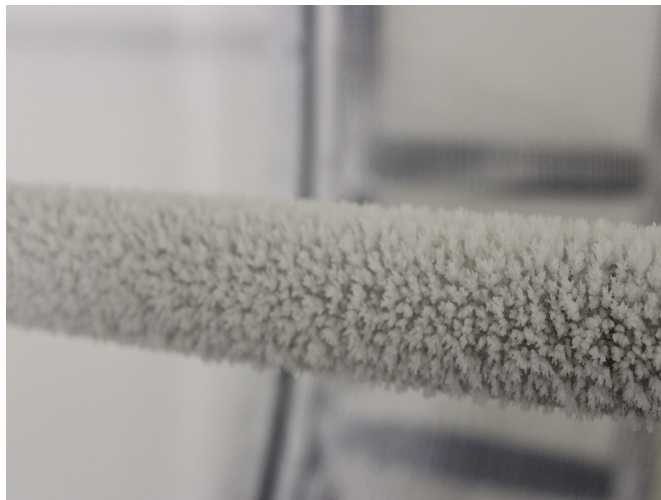
Figure 2-2: Soft rime on a conductor in the experiment
