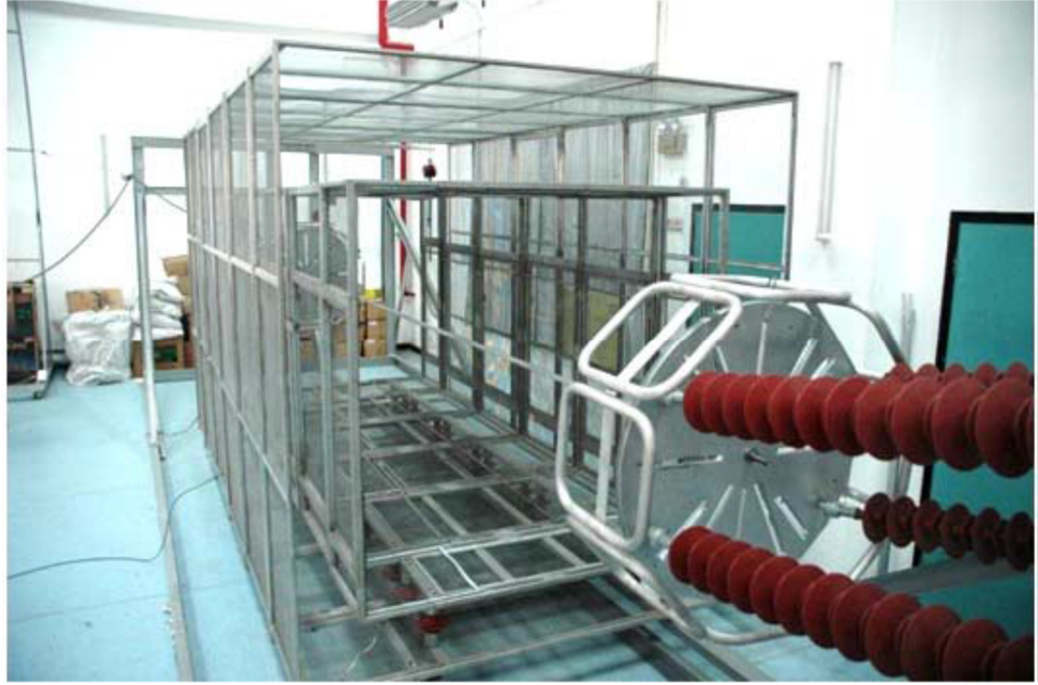
Figure 2-7: An indoor corona cage at Tsinghua University.
