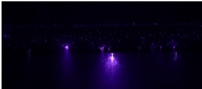
(b) Corona discharge of rime ice accreted conductor.
