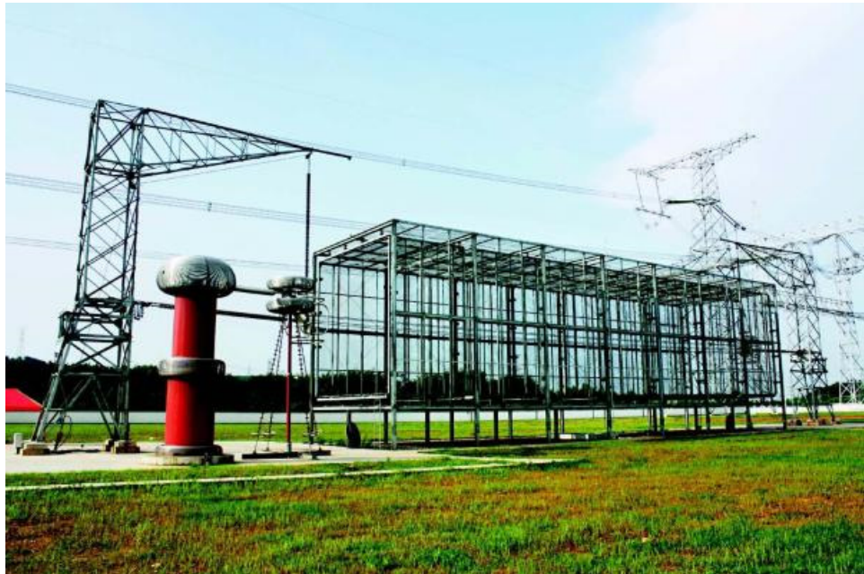
Figure 2-8: Outdoor corona cage at Wuhan Bureau of China Electric Power Research Institute.
