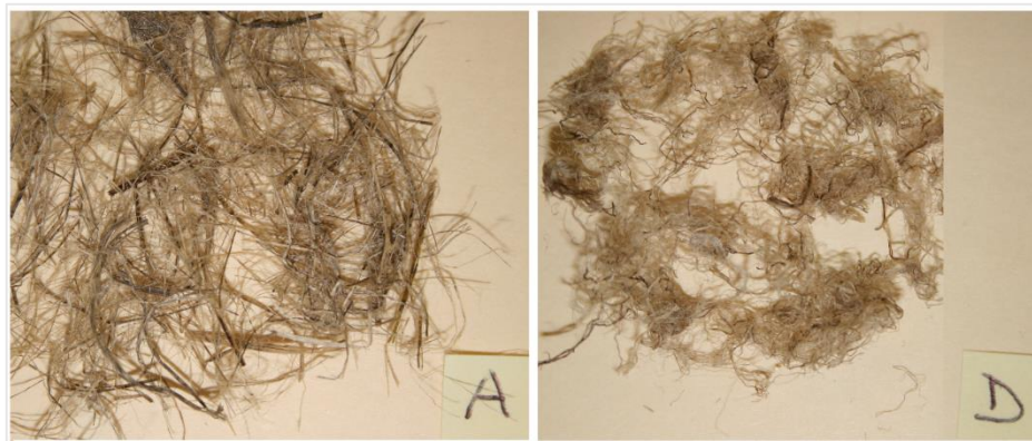
Figure 3-1: Aspect variation of hemp fibers: Virgin (A) and alkaline treated (D).
