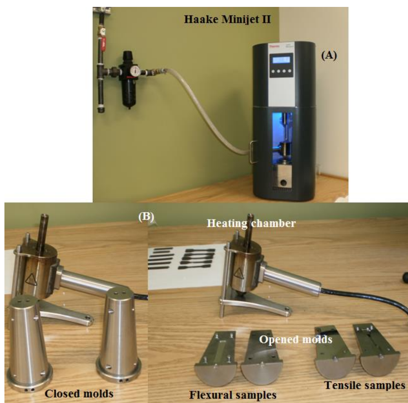
Figure 3-5: Mini injection molder, Haake Minijet II (A), its important parts, some flexural and tensional test samples (B).
