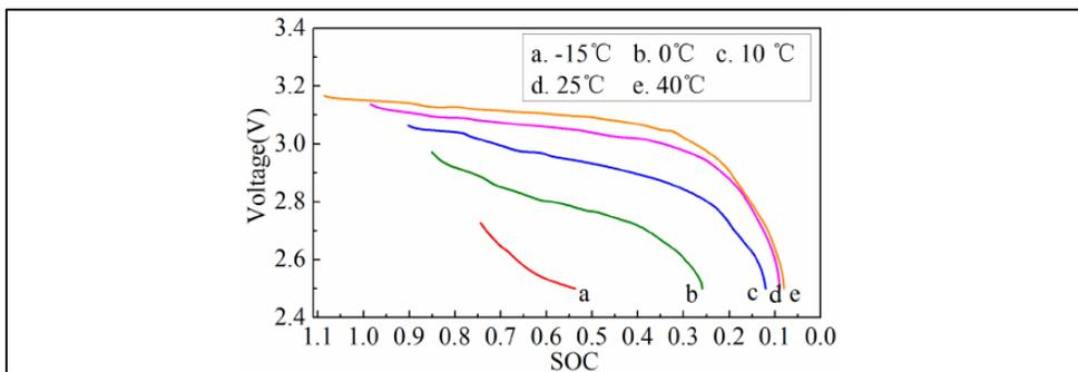
Figure 1-3 C-rate discharge curves of a LiFePO<sub>4</sub> cell at various temperatures
