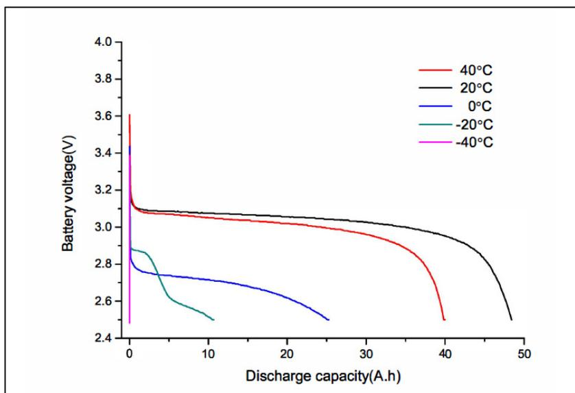
Figure 1-7 Discharging curves of 50A (1C) constant current under different temperatures
