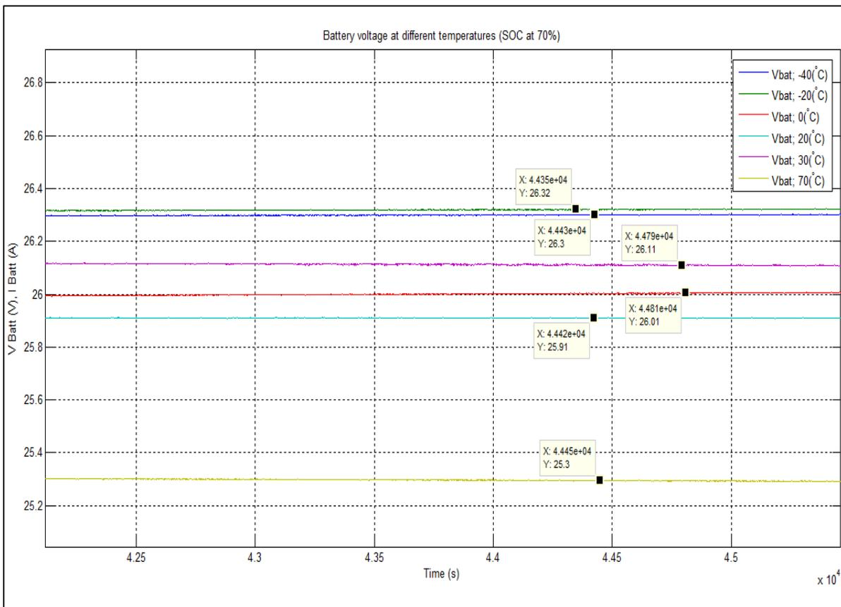
Figure 3-14 Battery voltage at different temperatures (SOC at 70%)
