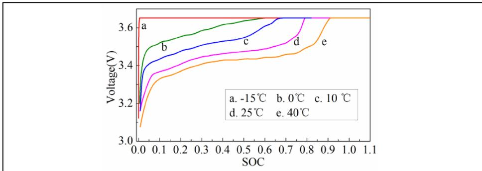
Figure 1-2 CCCV charge curves of a LiFePO<sub>4</sub> cell at various temperatures
