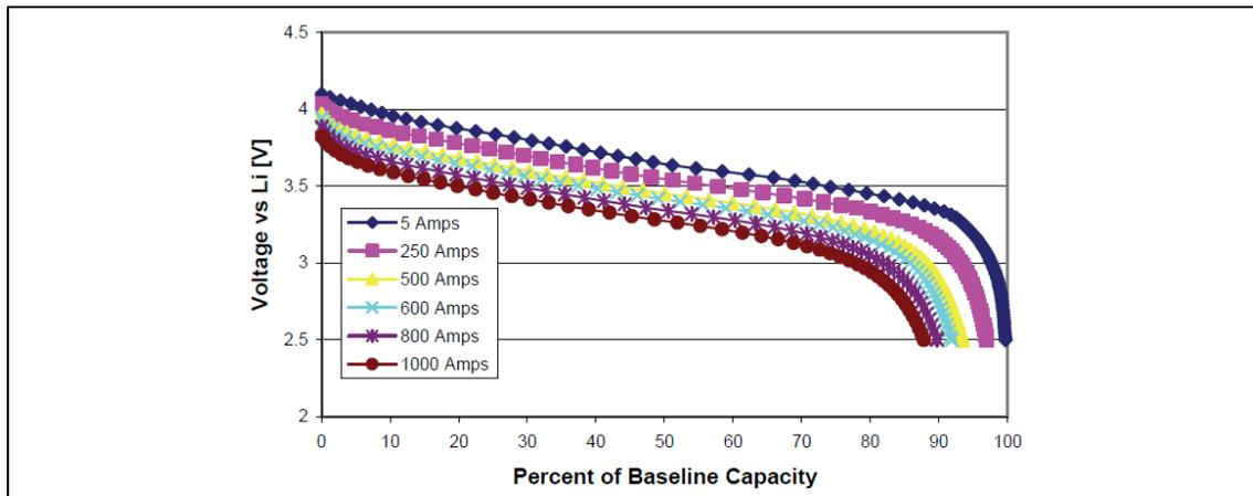
Figure 1-5 Discharge capacity at 60°C as a function of discharge rate. Saft Li-Ion cells
