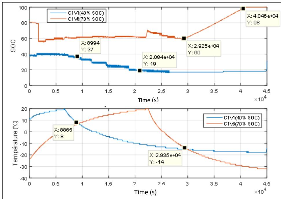
Figure 4-16 SOC unstable – S2 battery
