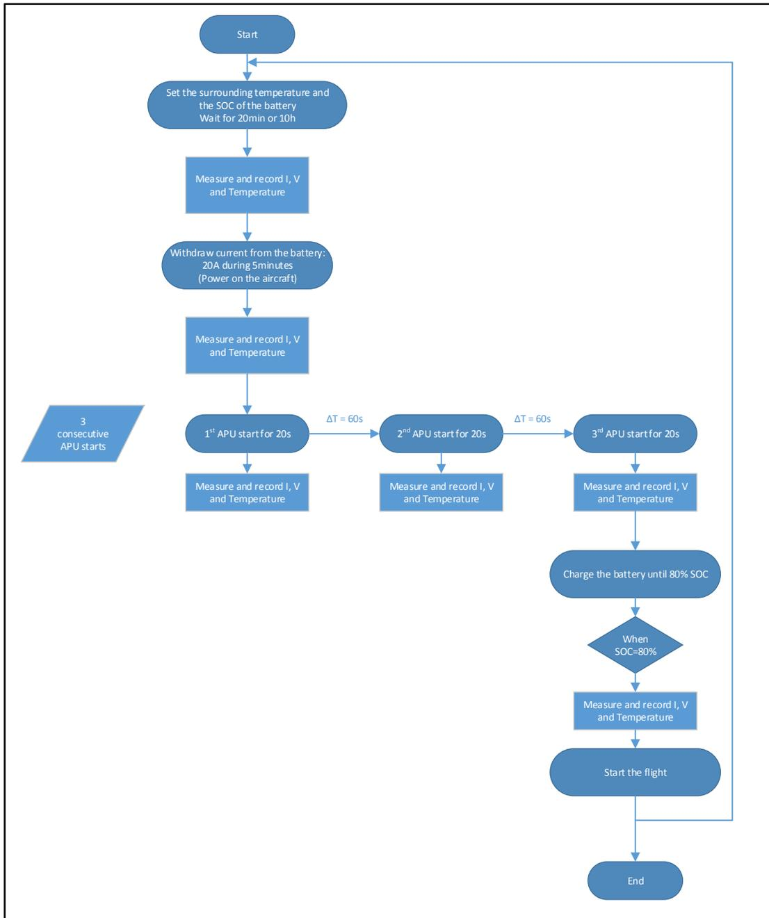
Figure 2-2 Algorithm of a flight simulation (Process to test the battery)
