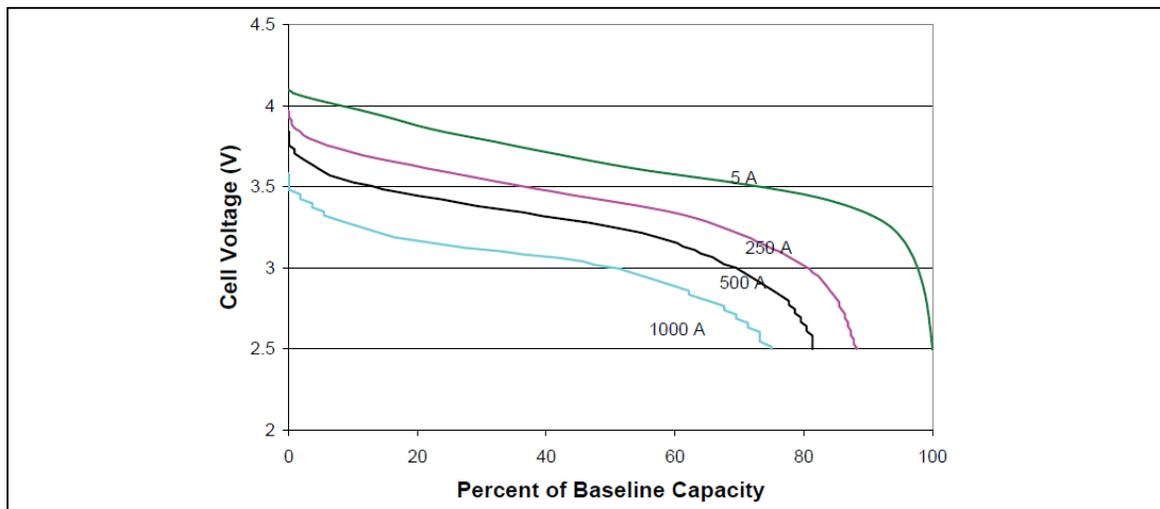
Figure 1-8 Voltage and discharge capacity as a function of rate of discharge at 20 °C
