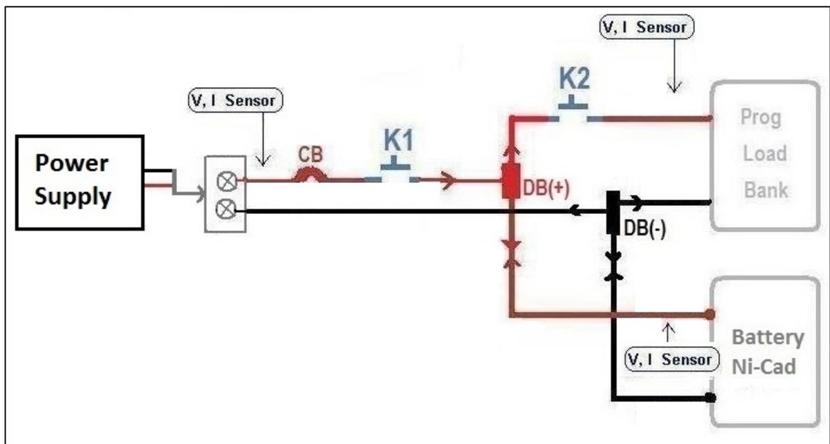
Figure-A I-1 Electrical wiring and sensors of the Ni-Cd bench test
