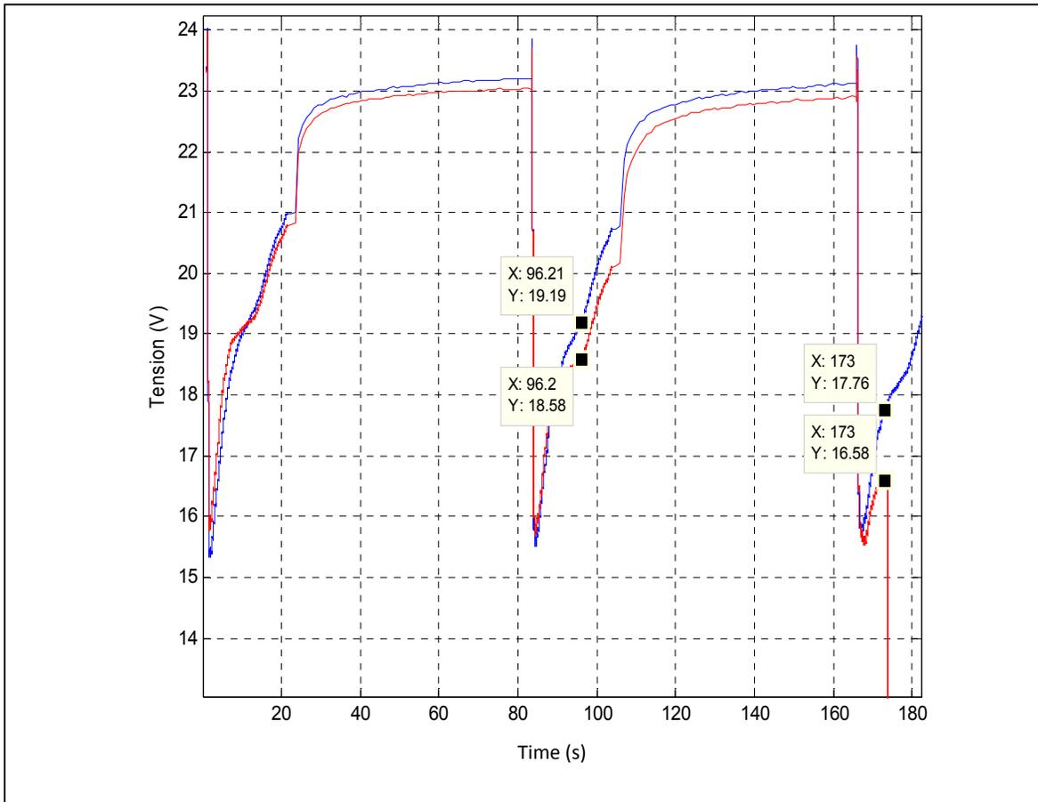
Figure 4-14 Voltage during APU, SOC at 40% and chamber temperature at  $-20^{\circ}\text{C}$
