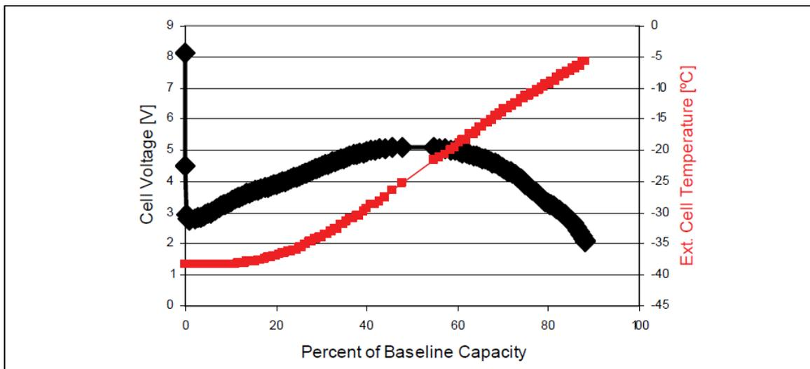
Figure 1-6 Discharge curve of two cells in series at  $-40^{\circ}\text{C}$  and 1000A (200C). The black curve is voltage and the red curve is exterior cell temperature. Cells: Saft UHP (VL5U)
