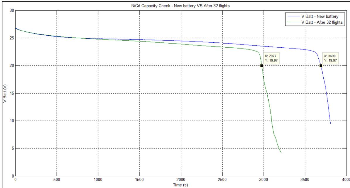
Figure 3-24 Capacity check- New battery VS After 32 flights
