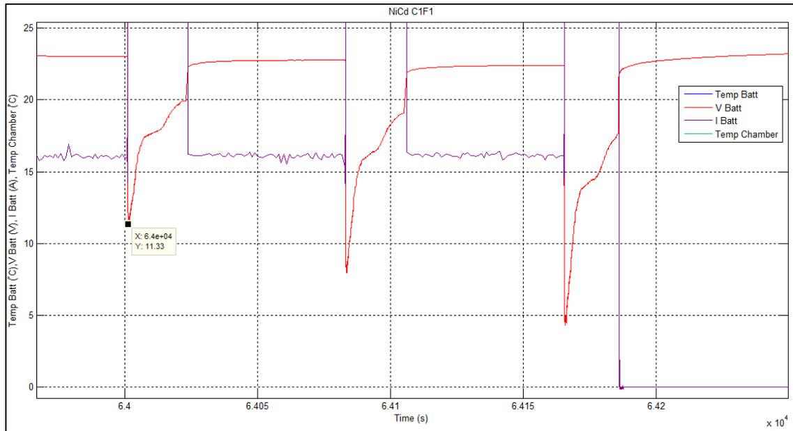
Figure 3-6 Voltage curve (red) of the first flight tested at -20°C and 40% SOC
