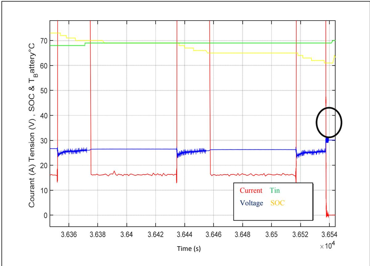
Figure 4-13 Test at 70°C with an SOC at 80%
