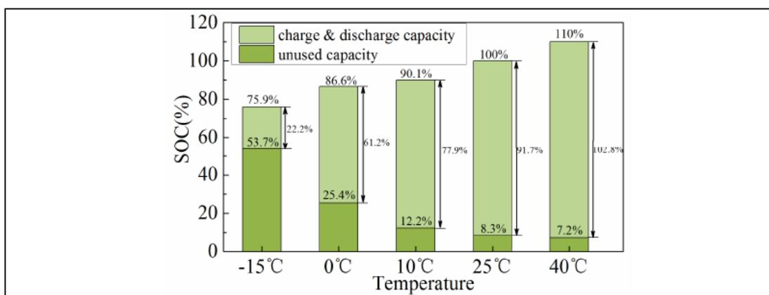
Figure 1-4 Charge and discharge capacity of a LiFePO<sub>4</sub> cell at various temperatures
