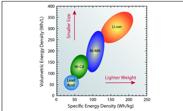
Figure 1-1 Comparison of the energy density of batteries
