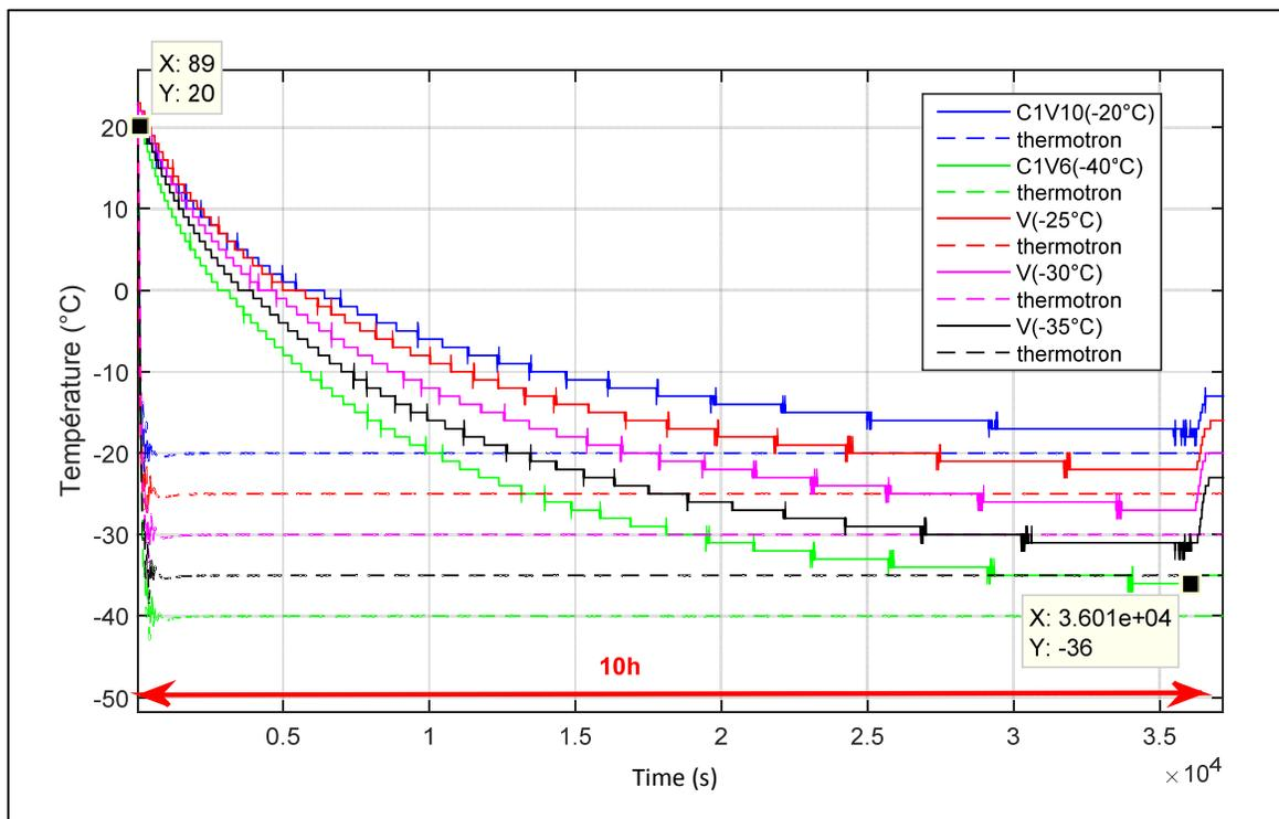
Figure 4-6 Thermal transfer at different temperatures (SOC at 70%)
