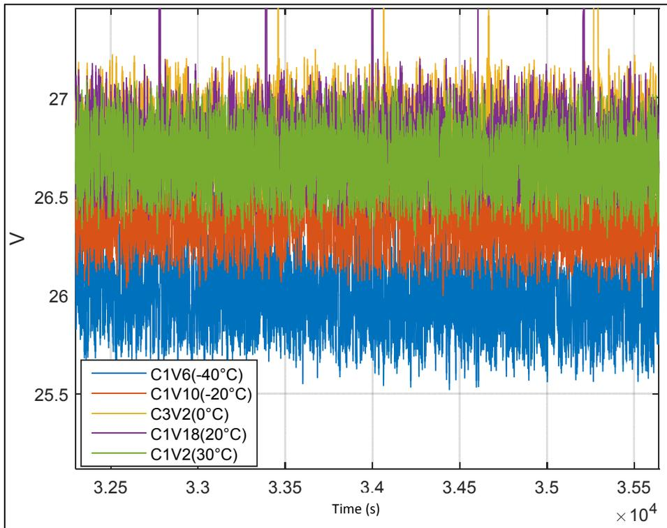
Figure 4-1 Battery voltage at different temperatures (SOC at 70%)
