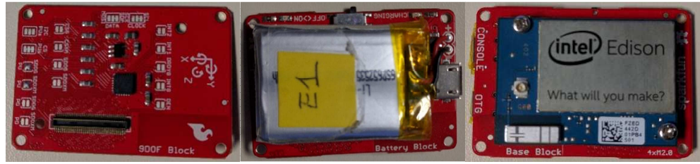
Figure 3: 9Dof Block (Left), Battery Block (Middle), Base block (Right).
