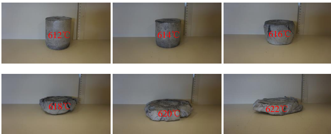
Fig. 4.22 Physical images of compressed billets by parallel plate viscometer at different temperatures of AA7075 base alloy
