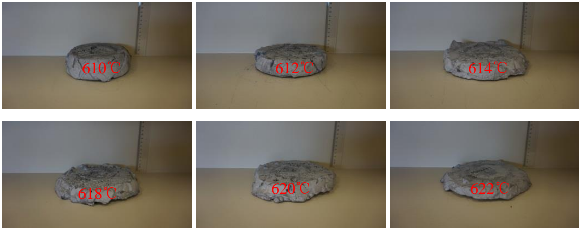
Fig. 4.30 Actual view of compressed billets by parallel plate viscometer at different temperatures of TiB 2 modified AA7075 alloy
