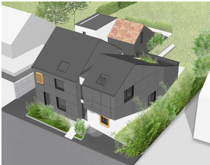
Figure 51: Calpinage de la façade (Source: Charlotte Dautremont)
