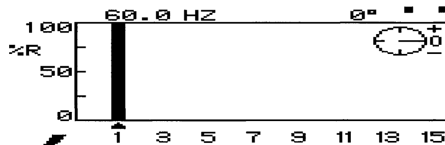
Figure 165 Spectre harmonique du courant source (THD=1.9%)
