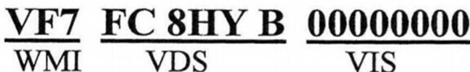
The diagram shows a VIN code 'VF7FC8HYB00000000' broken down into three sections. The first section 'VF7' is underlined and labeled 'WMI' below it. The second section 'FC 8HY B' is underlined and labeled 'VDS' below it. The third section '00000000' is underlined and labeled 'VIS' below it.
